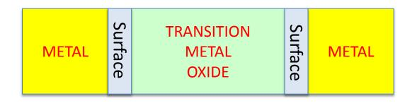
The surfaces are defect-rich with oxygen vacancies, transition metal excess, grain boundaries...
